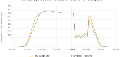
1 MW Energy Production Standard Tracking vs TrueCapture
